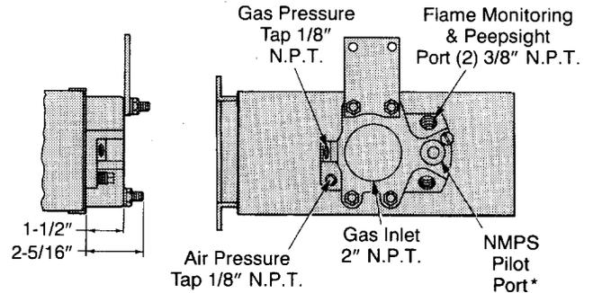
\*On casting #03877-1 for direct spark ignition of 6, 12, & 18 NML burners, this hole is tapped for spark plug #16927.
